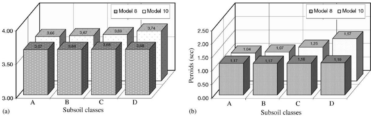
Fig. 13. Comparisons of the periods of (a) the convective mode and (b) impulsive mode for Models 8 and 10 according to subsoil class.
