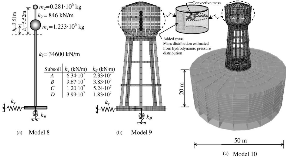
Fig. 12. Selected mechanical model and the finite element models for the soil–structure–fluid system.
