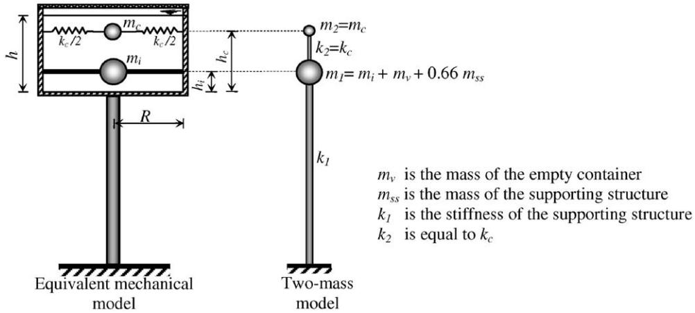
Fig. 3. Two-mass model for the elevated tanks suggested by Housner.
