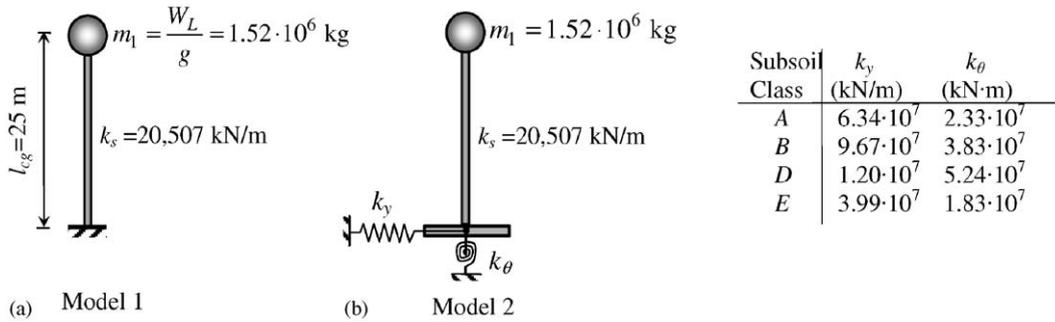
Fig. 9. The stiffness and mass values estimated for the single lumped-mass model of the elevated tank.
