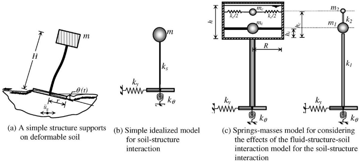
Fig. 4. Mechanical model for the fluid–structure–soil interaction of the elevated tank.
