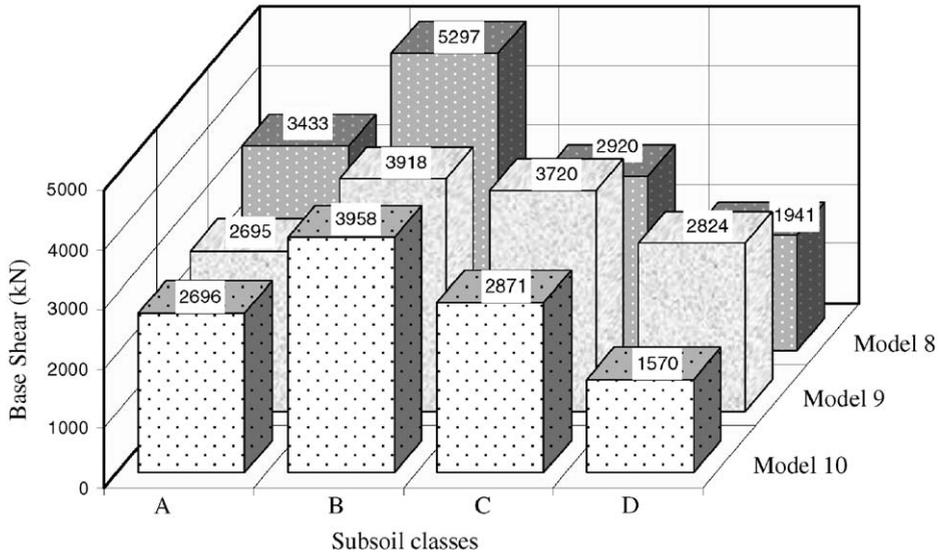
Fig. 14. Comparisons of the base shear forces for Models 8–10 according to subsoil class.
