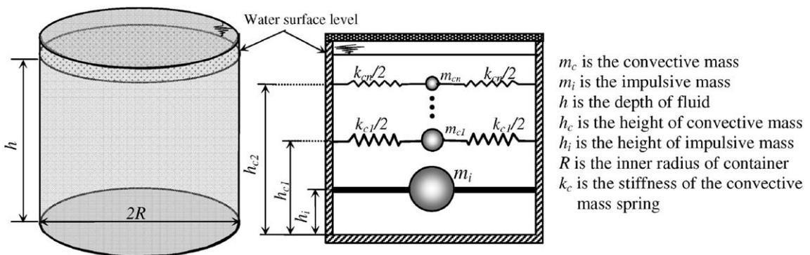
Fig. 2. Spring-mass analogy for ground supported cylindrical tanks.
