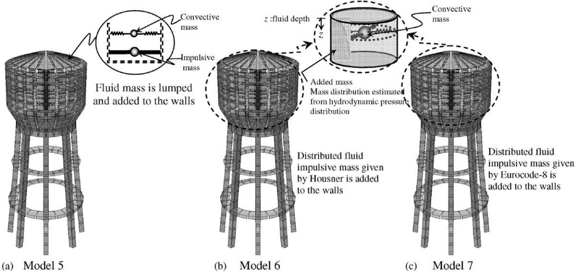
Fig. 11. Finite element mesh of the fluid–structure system for the added mass approach with the assumption of the fixed-base.
