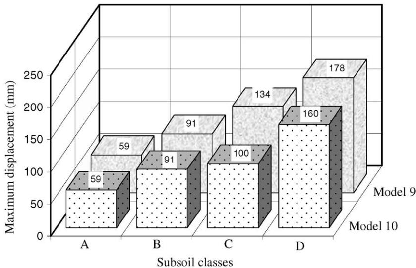
Fig. 15. Comparisons of the displacements for Models 9 and 10 according to subsoil class.
