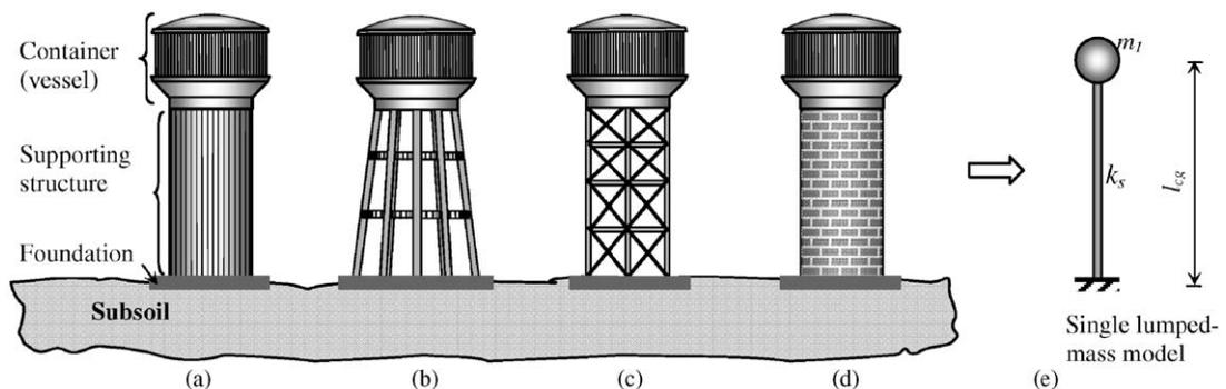
Fig. 1. Elevated tanks and the single lumped-mass model: (a) the tank with reinforced concrete shaft supporting structure, (b) the tank with reinforced concrete frame supporting structure, (c) the tank with reinforced concrete frame with diagonal braces or steel frame supporting structure, (d) the tank with masonry pedestal supporting structure, (e) single lumped-mass model.
