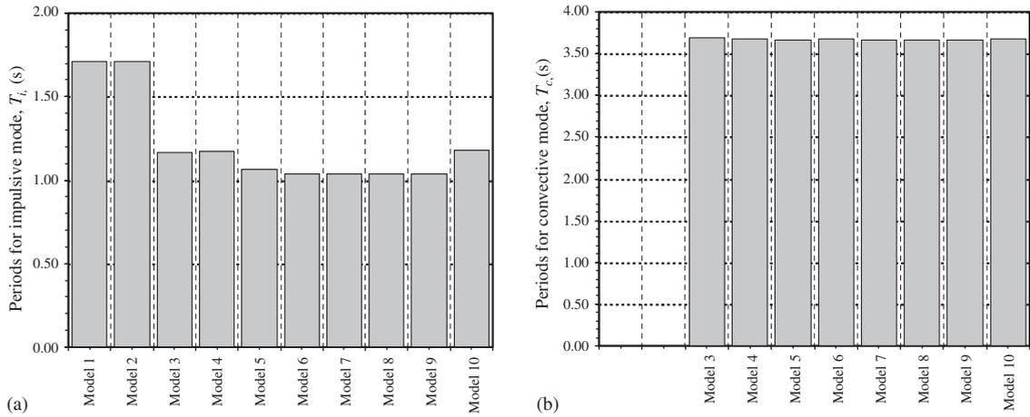
Fig. 16. Periods for (a) impulsive mode and (b) convective mode obtained for ten models considered for subsoil of class A.
