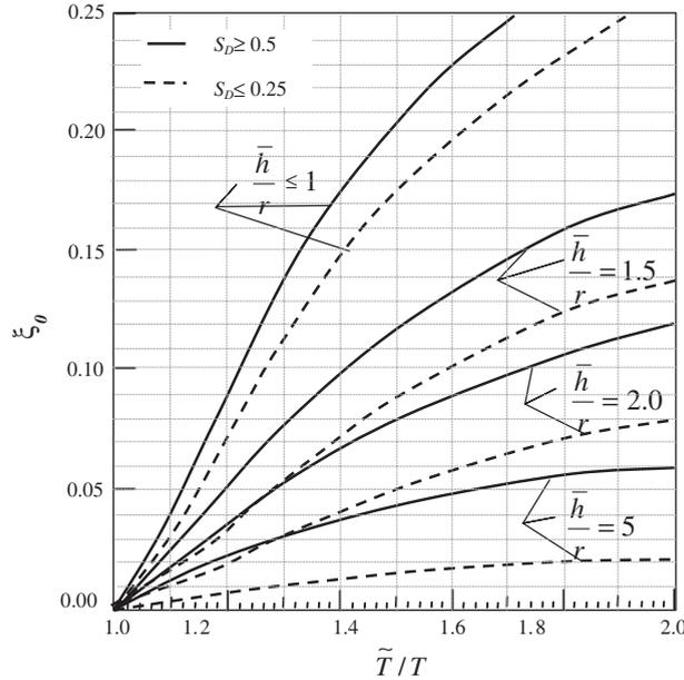
Fig. 5. Foundation damping factor (FEMA 368, 2000).
