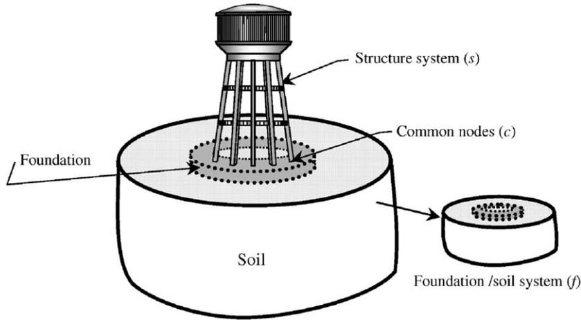
Fig. 6. Considered structure–foundation/soil interaction model.
