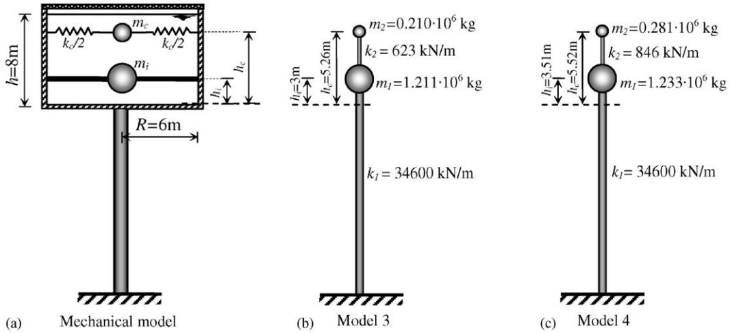
Fig. 10. The stiffness and mass values estimated for the two-mass model of Housner and Eurocode-8 with the assumption of fixed-base.
