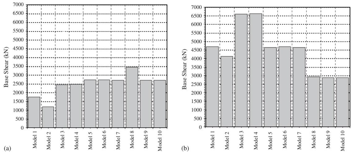
Fig. 17. Base shears obtained for ten models considered for subsoil of (a) class A and (b) class D.
