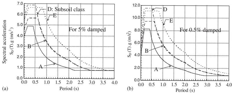
Fig. 8. Elastic response spectra of Type-1 recommended by Eurocode-8 for subsoil of classes A, B, D and E.
