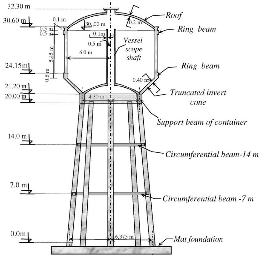
Fig. 7. Vertical cross-section of the reinforced concrete elevated tank considered for seismic analysis.
