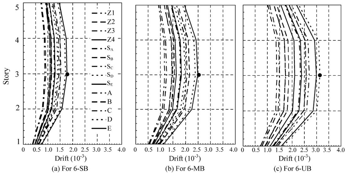
**Fig. 8** Drift for the 6-story buildings considering ground types defined in the codes
