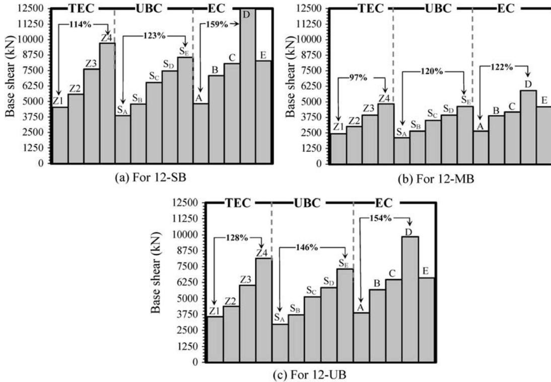
Fig. 7 Base shears for 12-story buildings considering fourteen ground types defined in the codes
