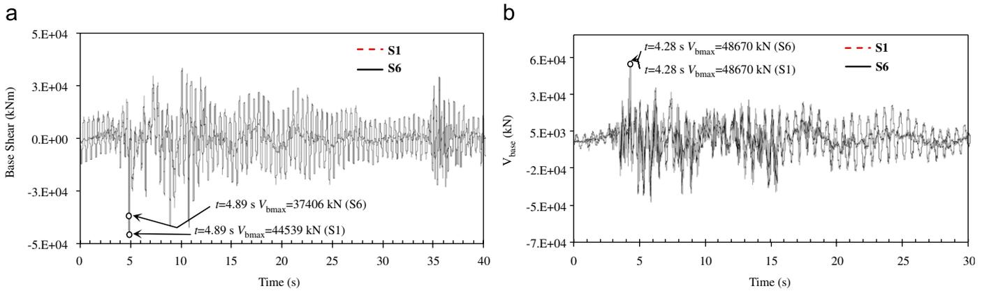
Fig. 15. Deviations of the base shear forces in time between the rigid-rectangular tank on S1 and S6 soil types for two ground motions of (a) Kocaeli (b) Düzce Earthquakes.
