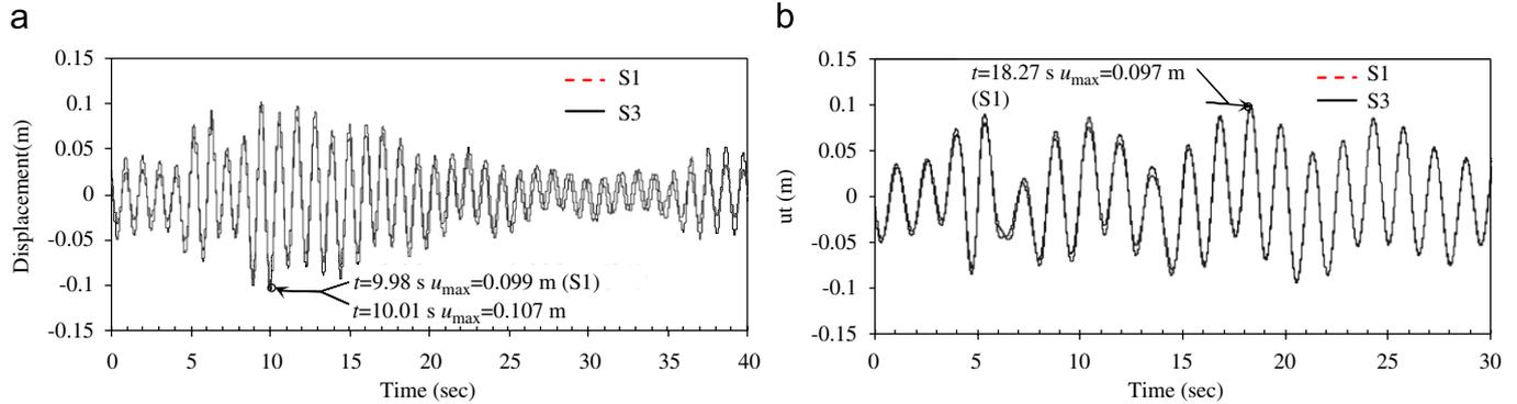
Fig. 9. Deviations of the displacements in time between the flexible rectangular tank on S1 soil type and S3 soil type for two ground motions of (a) Kocaeli (b) Düzce Earthquakes.
