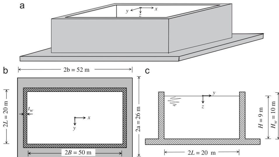
Fig. 7. Plan and elevation of the sample rectangular tank.
