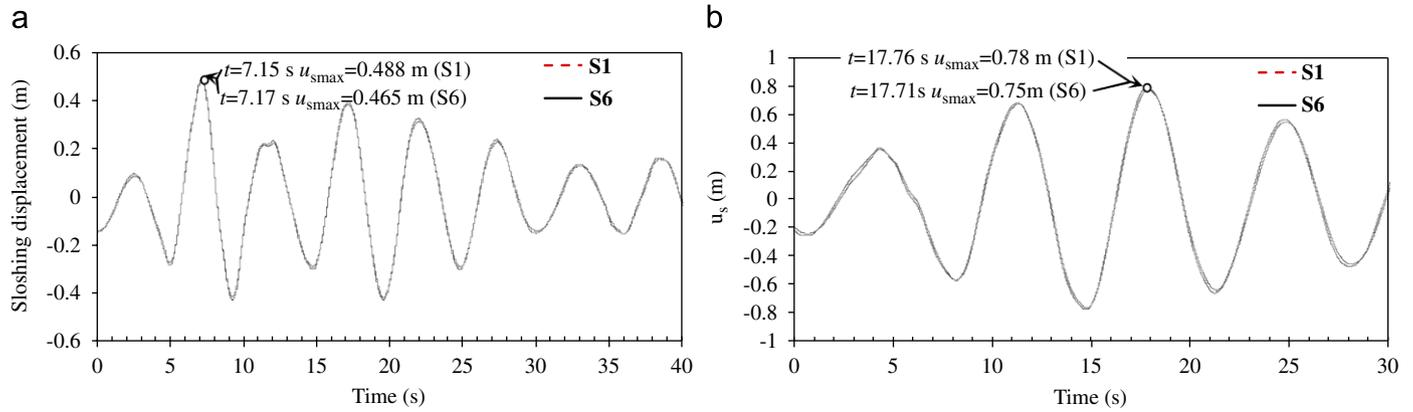
Fig. 12. Deviations of the sloshing displacements in time between the flexible tank on S1 and S6 soil types for two ground motions of (a) Kocaeli (b) Düzce Earthquakes.
