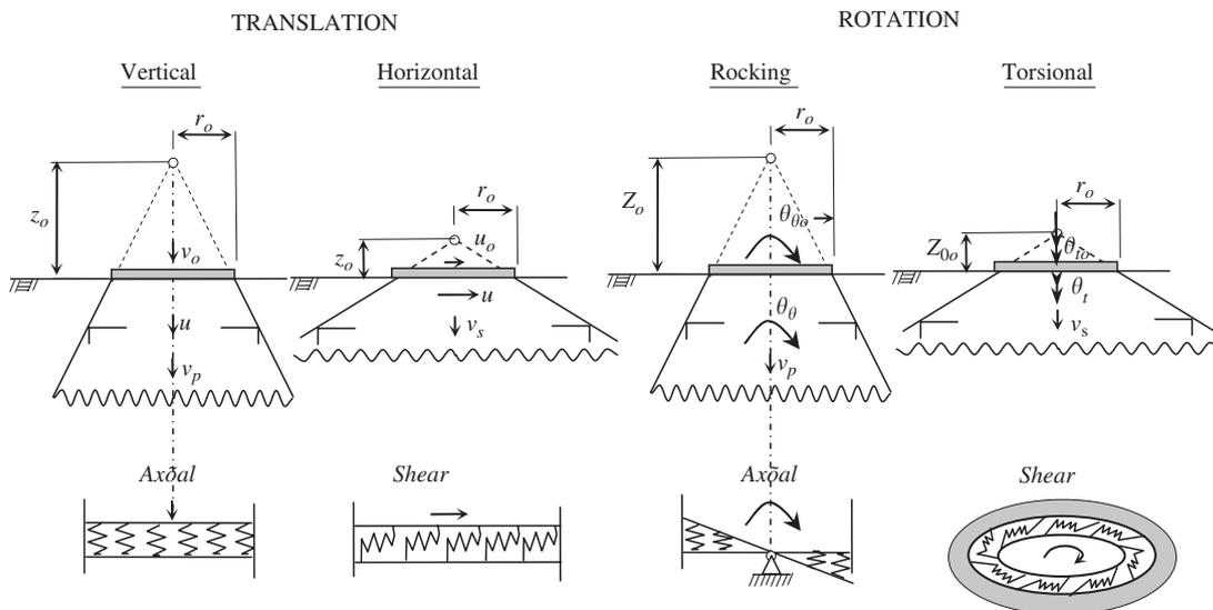
Fig. 3. Cones for various degrees-of-freedom with corresponding aspect ratio ( $z_0/r_0$ ), wave-propagation velocity and distortion [32,34]  $v_s$  and  $v_p$  are the shear and dilatational wave velocities.
