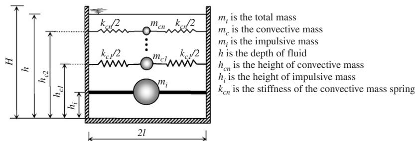
Fig. 2. The equivalent spring-mass model of the fluid.
