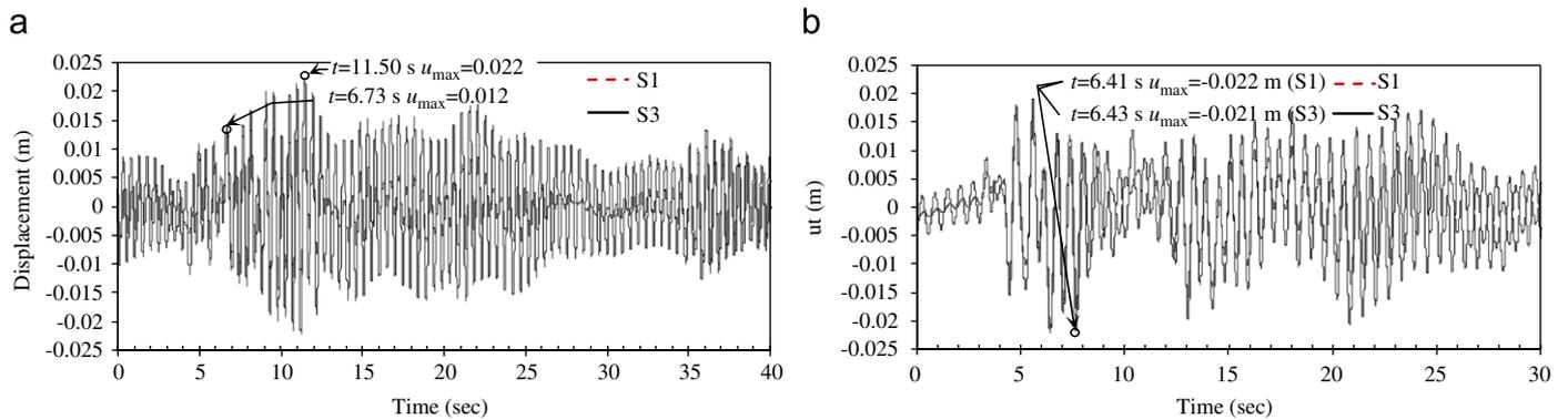
Fig. 10. Deviations of the displacements in time between the rigid-rectangular tank on S1 soil type and S3 soil type for two ground motions of (a) Kocaeli (b) Düzce Earthquakes.
