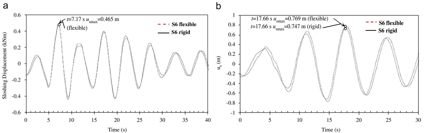
Fig. 16. Deviations of the sloshing displacements in time between the flexible rectangular tank and rigid tank on S6 soil type for two ground motions of (a) Kocaeli (b) Düzce Earthquakes.
