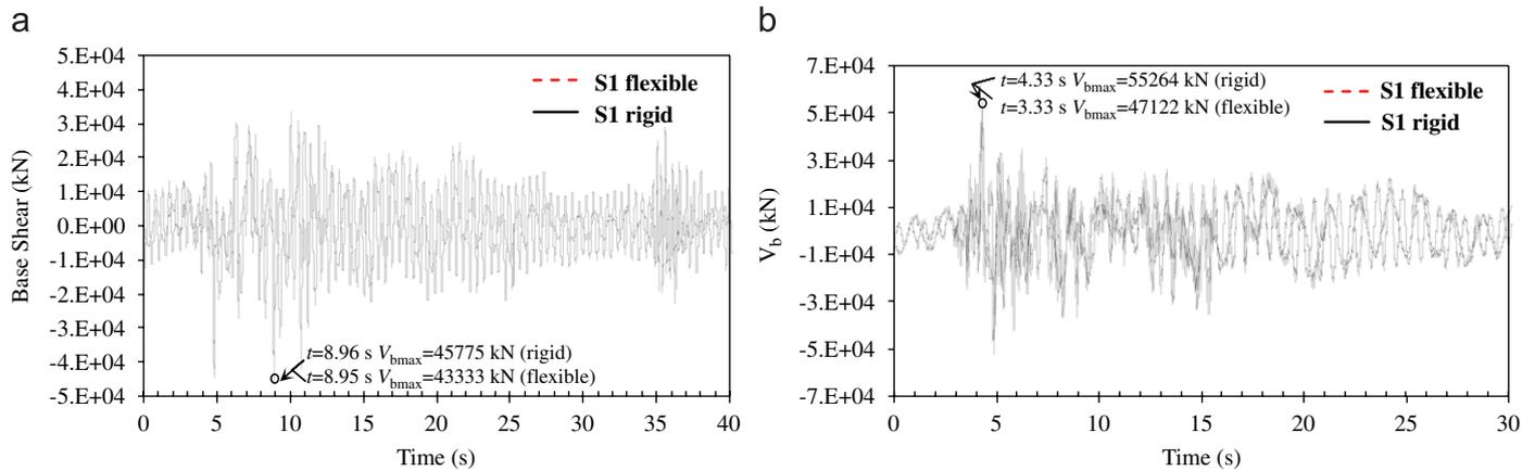
Fig. 17. Deviations of the base shear forces in time between the flexible rectangular tank and rigid tank on S1 soil type for two ground motions of (a) Kocaeli (b) Düzce Earthquakes.
