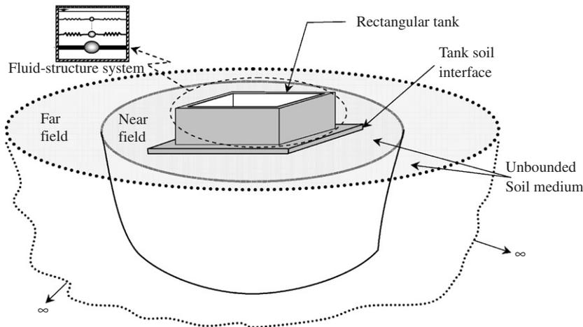
Fig. 1. The problem investigated for dynamic fluid–rectangular tank–soil interaction.
