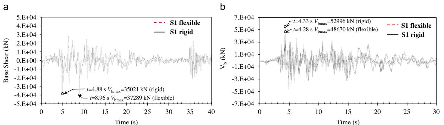
Fig. 18. Deviations of the base shear forces in time between the flexible rectangular tank and rigid tank on S6 soil type for two ground motions of (a) Kocaeli (b) Düzce Earthquakes.
