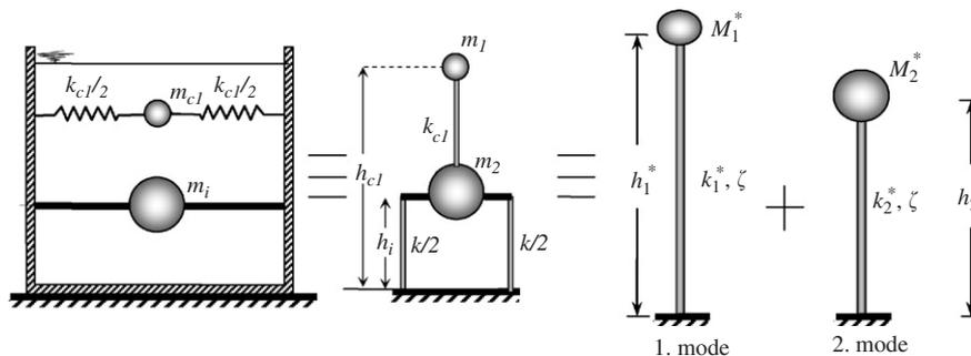
Fig. 5. Two mass model represented by two mode properties of the elevated tank.
