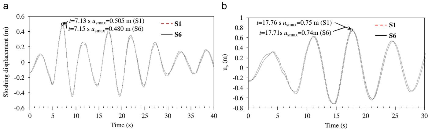
Fig. 13. Deviations of the sloshing displacements in time between the rigid tank on S1 and on S6 soil types for two ground motions of (a) Kocaeli (b) Düzce Earthquakes.
