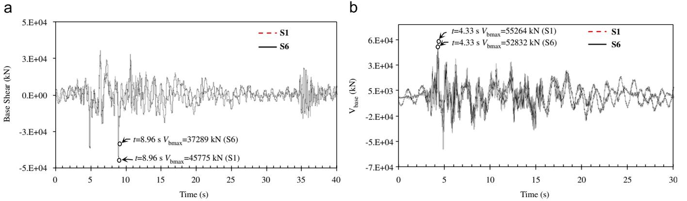
Fig. 14. Deviations of the base shear forces in time between the flexible rectangular tank on S1 and S6 soil types for two ground motions of (a) Kocaeli (b) Düzce Earthquakes.
