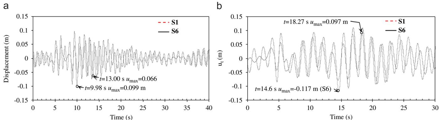
Fig. 11. Deviations of the displacements in time between the flexible rectangular tank on S1 soil type and S6 soil type for two ground motions of (a) Kocaeli (b) Düzce Earthquakes.
