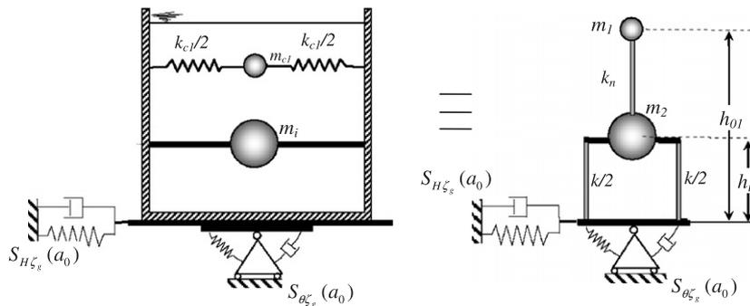
Fig. 4. Considered mechanical model for the fluid–rectangular tank–soil/foundation system.
